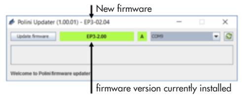
When you connect the USB cable without switching the battery on, the following screen will be displayed:
