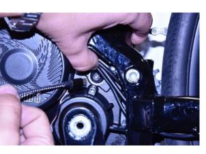
Connect the micro USB cable to the motor (be careful to the way of connection) and the USB plug to a PC with Window 7 installed or latest versions.
