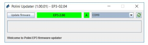
When the COM is selected and the communication is active, the firmware version currently installed is visible inside the green bar.
