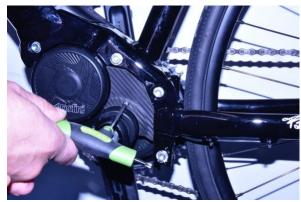
Remove the plastic cover using a Torx 20 key
