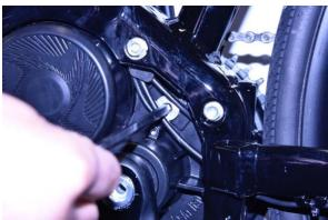
Remove the aluminum cap using a CH6 a hex key
