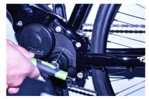
Using a Torx 20 key remove the plastic cover
