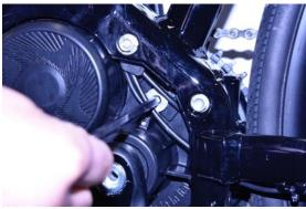
Remove the aluminum cap using an Allen key CH6
